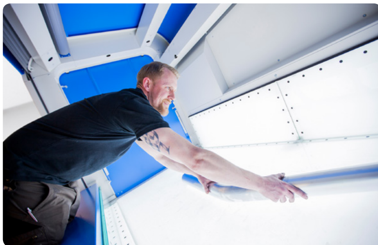
→ Stefan Chestersson puts a tube into TubeInspect P16. The new narrow front edge allows for an ergonomically optimized insertion of measuring objects into the measuring cell. (Image: Proton Group)
